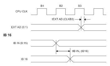
Note: All time measurements on active signals relate to 1.5V levels.
