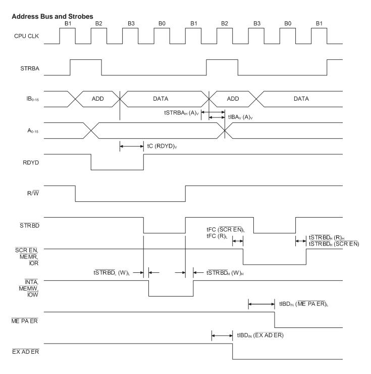
Note: All time measurements on active signals relate to 1.5V levels.
