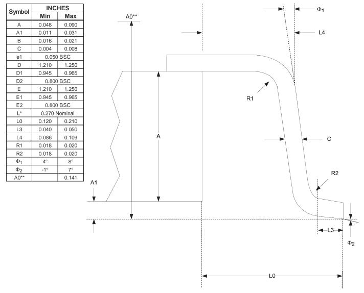
\* Lead length in the straight lead configuration, prior to leadforming (used for all test and in-process WIP operations).
