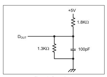
Figure 1. Output Load
